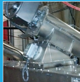
Binswitch Installed on Bucket Elevator Spouting (with SMP, BAS & conduit adapter)
